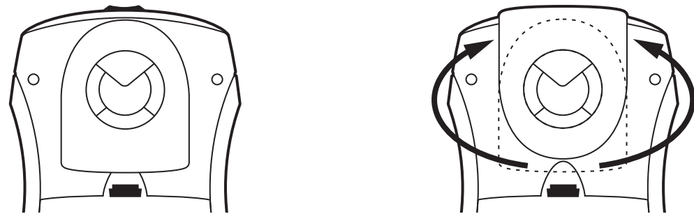
Figure K1: R35-8 Belt Clip Installation Figure K2: Turn Belt Clip
