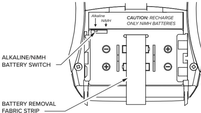
1. **Install the AA batteries.** Be sure to observe proper polarity (+/-). Damage due to improper battery installation may void the warranty on the product.
