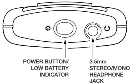
6. Plug in the earphones/headphones into the headphone jack (Figure 8). The earphone/headphone cord functions as the antenna.
