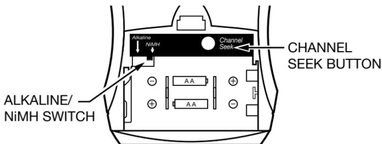
5. To lock or unlock a selected channel, turn the power off. While holding the seek button, turn the power back on. When locked, the receiver will remain on the current channel, regardless of channel seek button presses.
