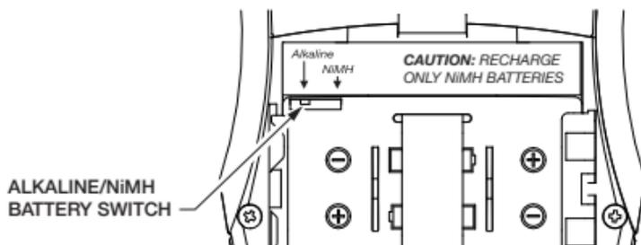
2. Install the AA batteries. Be sure to observe proper polarity (+/-). Damage due to improper battery installation may void the warranty on the product. The “Power On” LED on top of the unit will flash when the batteries are getting low; you may continue to use until the unit quits operating, then replace or recharge the batteries. (FIG. A)
