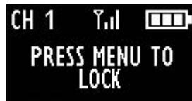
When the display shows “PRESS MENU TO LOCK”, release the buttons. Then push the Menu button to lock. The display will show “LOCKED” (below) and then will return to the home screen.
