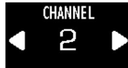
Push either arrow button to **step** to one of the 17 channels (above) -or- push-and-hold either arrow button to **seek** to the next active channel (below). The receiver is seeking the next *frequency*, so channels may appear out of order when seeking.
