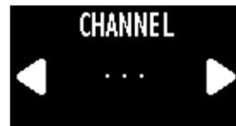
If no actively-broadcasting channels are found during the seek, a message is displayed (below). Make sure you are on the same channel as the transmitter. When finished, push the menu button once to get back to the home screen, and go to step 3.
