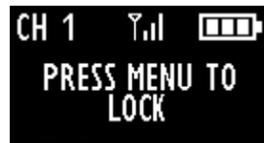
When the display shows PRESS MENU TO LOCK, release the buttons. Then push the Menu button to lock. The display will show LOCKED (below) and then will return to the home screen.
