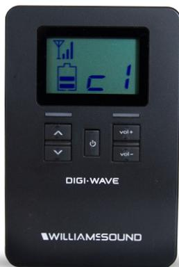
The DLR 400 ALK uses 2 AAA alkaline batteries rather than a rechargeable battery like the DLR 400 RCH.
