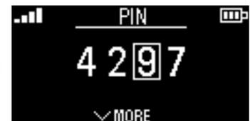
The same four digit code must be programmed into all of the Digi-Wave devices in the group. If a different secure code has been entered, participants cannot re-enter the group without re-entering the correct secure code. The only time the Encryption PIN is displayed is when it is being entered. As the PIN is being entered, individual numbers will be replaced by the \* symbol.
