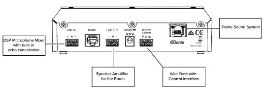
Speakers, Microphones and Other Components Your existing sound system can be connected to the BluePOD® Solo via the Dante port or via the Line In and Line Out Phoenix style connectors on the controller.
