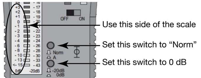
In the center of the loop, about 5 feet above the floor, measure the field strength with the meter. It will most likely read less than 0 dB. Go back to the amplifier and adjust the "Volume" level up. Go back to the loop, and with the field strength meter, measure the field strength again.
