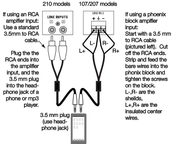
If using a phoenix block amplifier input: Start with a 3.5 mm to RCA cable (pictured left). Cut off the RCA ends. Strip and feed the bare wires into the phoenix block and tighten the screws on the block. L-,R- are the shields, L+,R+ are the insulated center wires.
