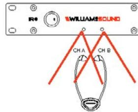
Tune the receiver to the IR Baseband channel the audio is playing on to ensure all your settings sound correct. This audio will match the audio from the IR E4 emitters.
