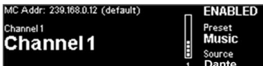
On the main menu, highlight a channel's VU meter and press and hold the right arrow to view additional information. Some channel settings can be edited. Use the up and down arrows to disable or enable the channel, or adjust the input source.
