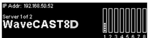
The main screen of the front panel displays the name of the server, the number of WaveCAST EIGHT D servers on the network, the IP address, and a VU meter for each channel.
