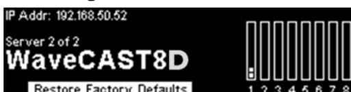
Restore Factory Defaults is a hidden option underneath the device name. Selecting this option will reset the device to its factory settings, including network and login settings for the Web Control Interface. Two confirmation prompts will appear before the settings are reset, including one to press down to confirm the restoration.
