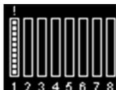
When a channel's audio is overloaded, an exclamation point will appear over that channel's VU meter. Adjust the audio for that channel to fix the issue. If no network connection is available, the VU meters may not function, even when audio is playing.
