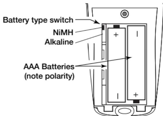
2. Insert two AAA NiMH batteries. Be sure to follow correct polarity (Figure 1). Do not use with alkaline batteries.
