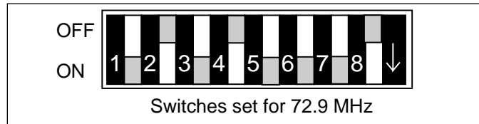
FIGURE 6: SETTING THE T17 FREQUENCY SELECTOR SWITCHES
