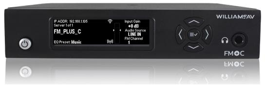
The new FM+ C transmitter integrates professional WaveCAST Wi-Fi audio server technology into a FM assistive listening system. Users can now listen with either an FM receiver or our dedicated WF R1/WF R2 receiver, or with their own smartphone (via the WaveCAST Receiver App). Venues no longer need to choose between providing FM or Wi-Fi assistive listening systems. Along with this flexibility comes exceptional audio quality, as the FM+ C is built on a DSP.
