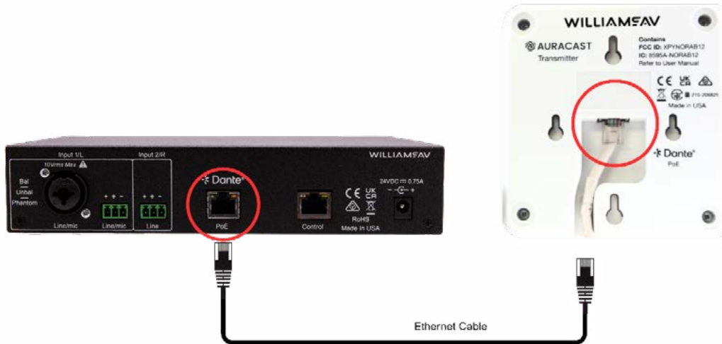
Figure 9: The Infinium Controller to Transmitter direct connection
